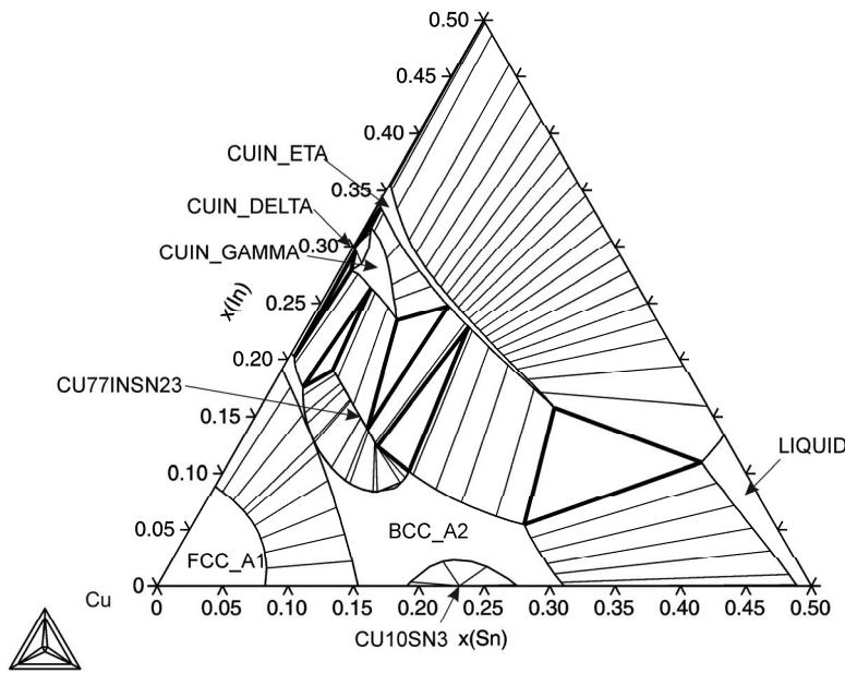
**Fig. 194:** Cu-rich corner of the isothermal section at 600 °C
