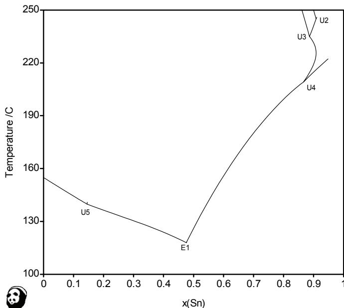
**Fig. 208:** Liquidus lines in the In-Sb-Sn system in the region of the low-temperature invariants projected onto the T- $x(\text{Sn})$  plane
