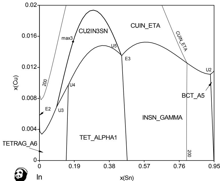
**Fig. 189:** Liquidus lines in the region close to the In-Sn binary edge in the Cu-In-Sn system
