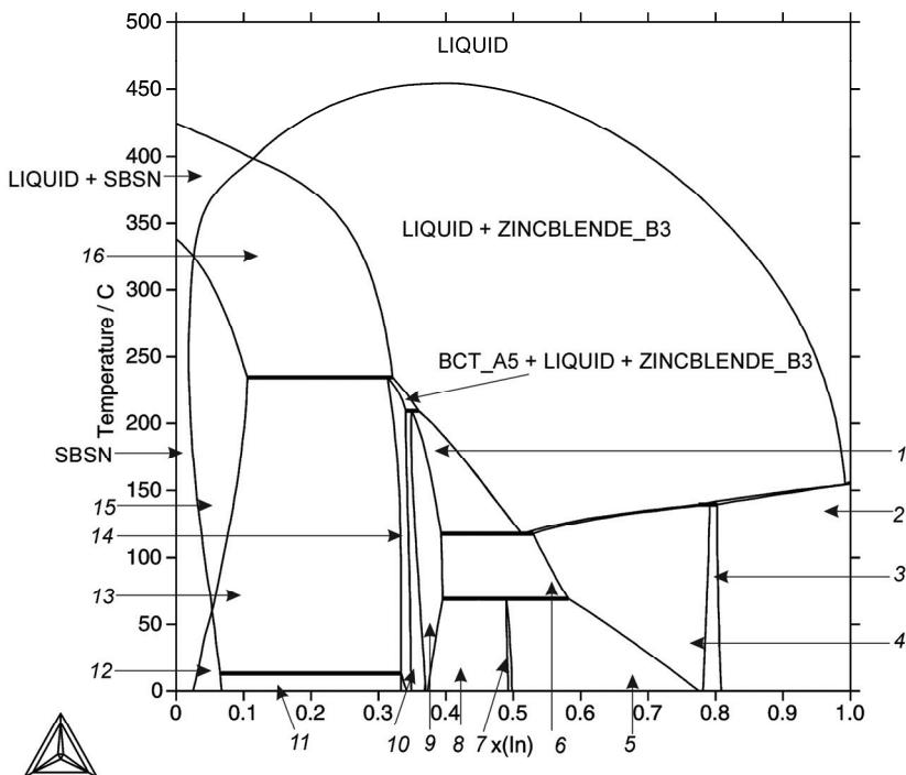
**Fig. 213:** Isopleth of the In-Sb-Sn system with the ratio Sb:Sn of 1:1
