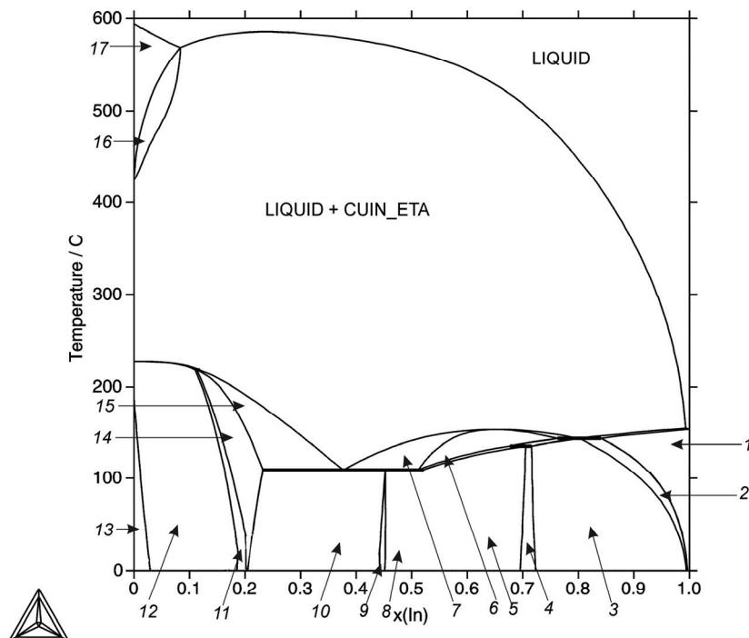
**Fig. 195:** Isopleth of the Cu-In-Sn system with the ratio Cu:Sn of 1:1
