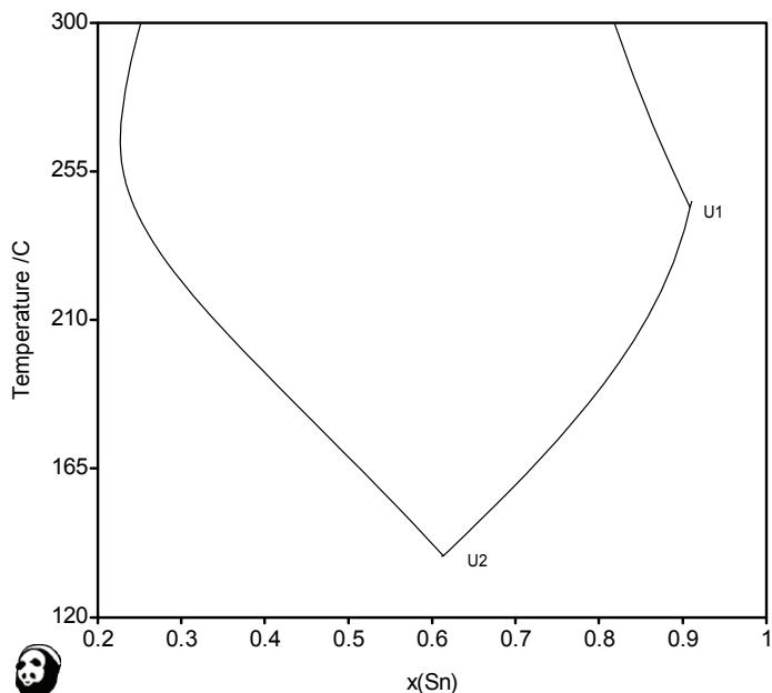
**Fig. 175:** Liquidus lines in the Bi-Sb-Sn system in the region of the low-temperature invariants projected onto the T- $x(\text{Sn})$  plane
