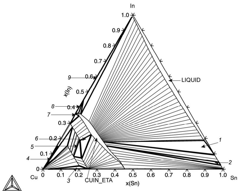
**Fig. 192:** Isothermal section at 200 °C
