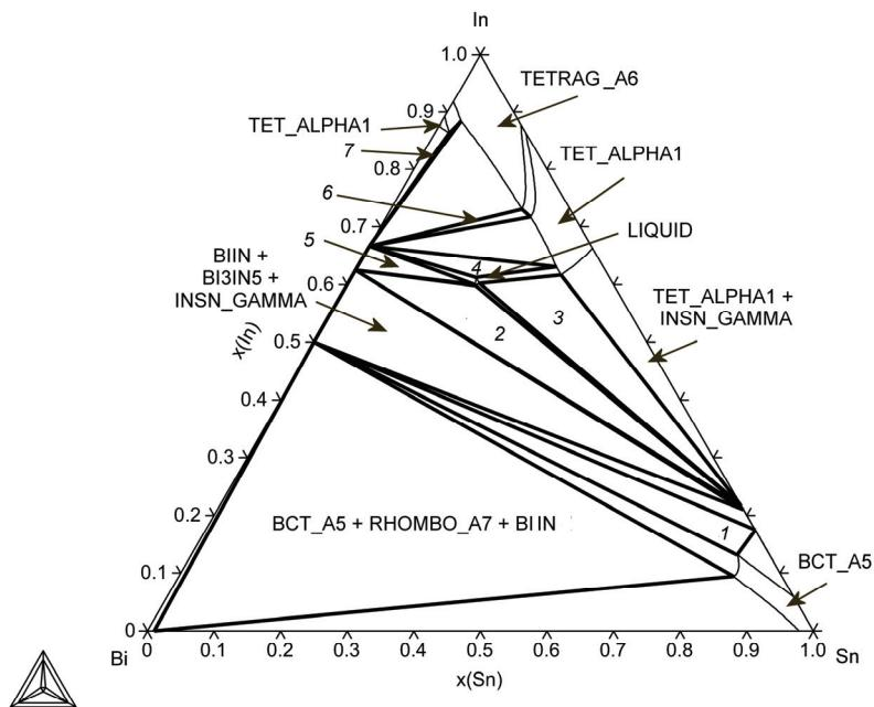
**Fig. 171:** Isothermal section at 56 °C
