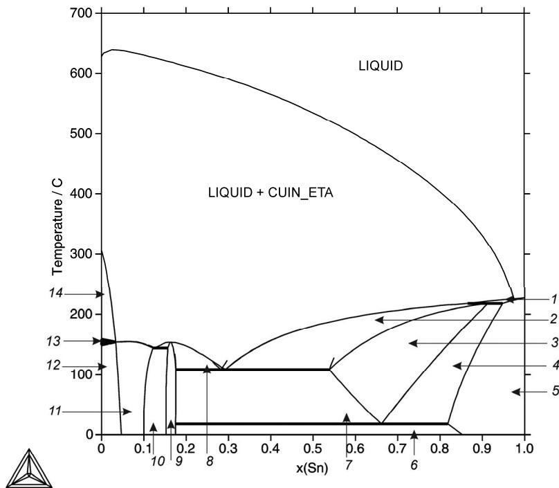
**Fig. 196:** Isopleth of the Cu-In-Sn system with the ratio Cu:In of 1:1
