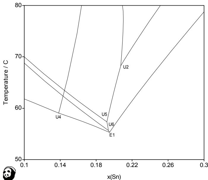
**Fig. 170:** Liquidus lines in the Bi-In-Sn system in the region of the low-temperature invariants projected onto the T- x(Sn) plane
