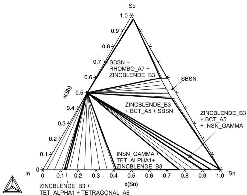
**Fig. 209:** Isothermal section at 100 °C
