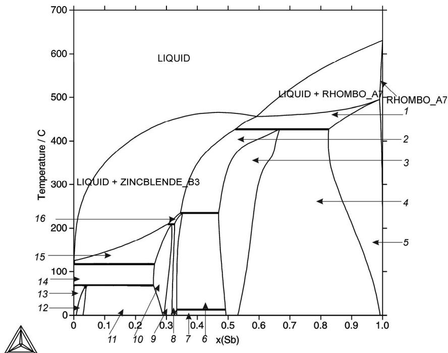
**Fig. 212:** Isopleth of the In-Sb-Sn system with the ratio In:Sn of 1:1
