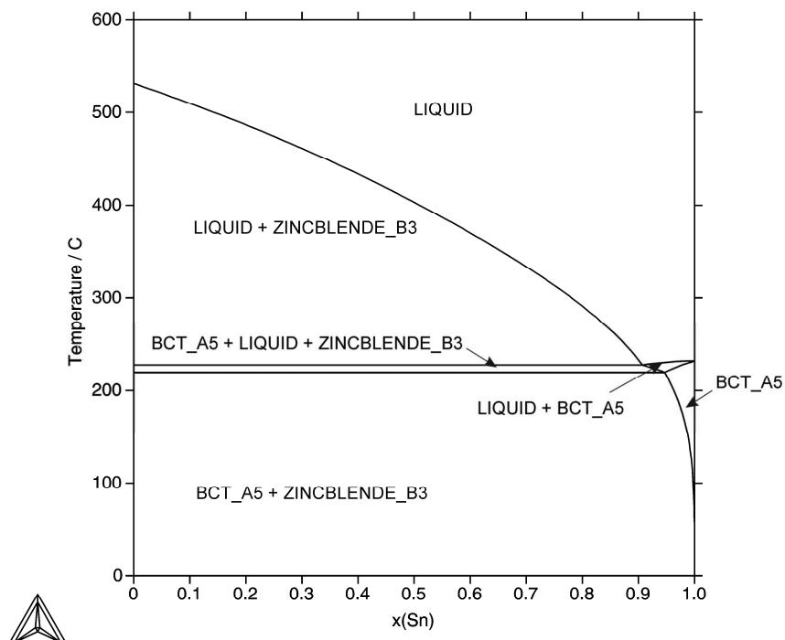
**Fig. 211:** Isopleth of the In-Sb-Sn system with the ratio In:Sb of 1:1
