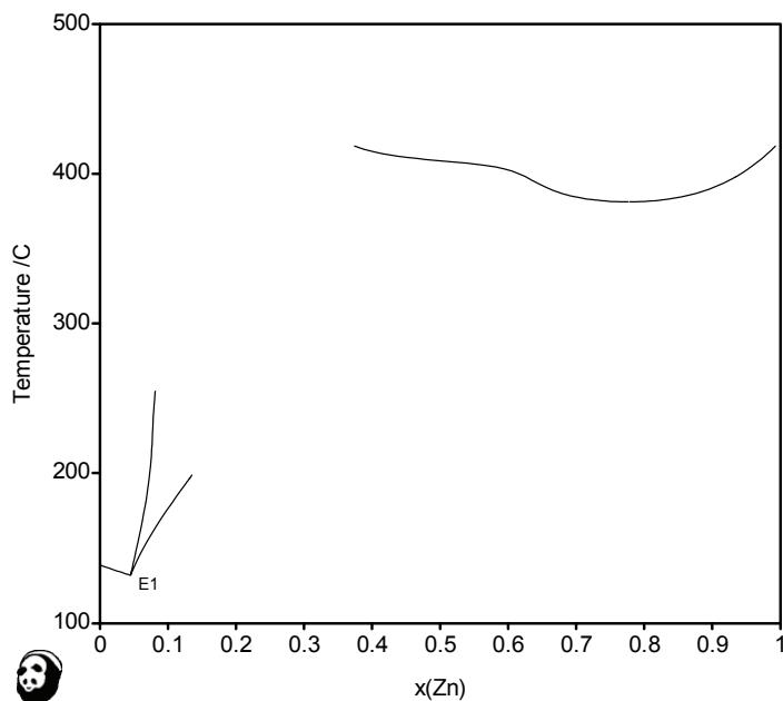
**Fig. 182:** Liquidus lines in the Bi-Sn-Zn system in the region of the low-temperature invariants projected onto the T- $x(\text{Zn})$  plane
