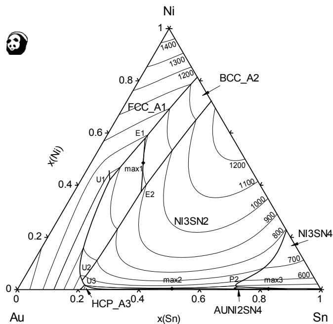
**Fig. 159:** Liquidus projection of the Au-Ni-Sn system
