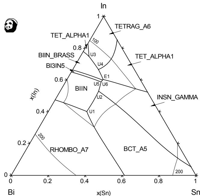
**Fig. 169:** Liquidus projection of the Bi-In-Sn system
