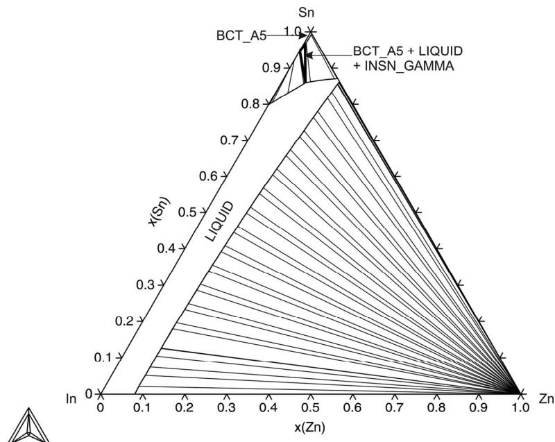
Fig. 217: Isothermal section at 200 °C
