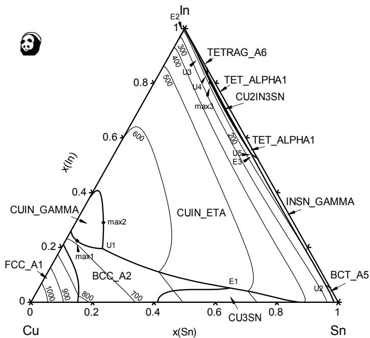
**Fig. 187:** Liquidus projection of the Cu-In-Sn system
