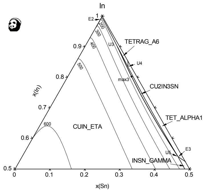
**Fig. 188:** Liquidus projection for the In rich corner of the Cu-In-Sn system
