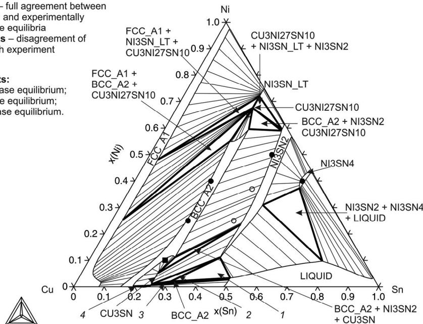
**Fig. 201:** Calculated isothermal section at 600 °C (compared with exp. data from [08Sch] obtained in the scope of COST 531 Action)
