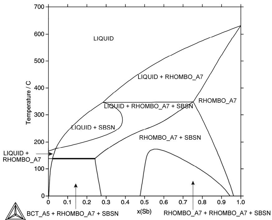
**Fig. 178:** Isopleth of the Bi-Sb-Sn system with the ratio Bi:Sn of 1:1
