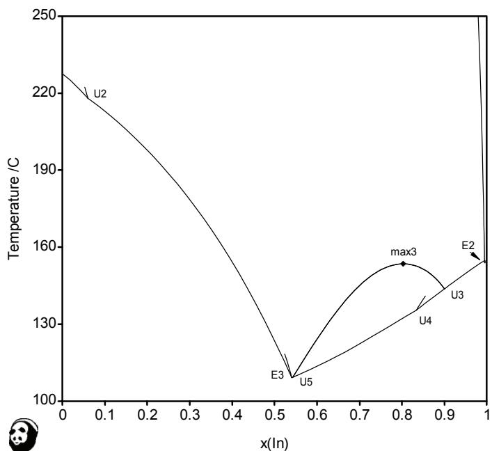
**Fig. 191:** Liquidus lines in the Cu-In-Sn system in the region of the low-temperature invariants projected onto the T- $x(\text{In})$  plane
