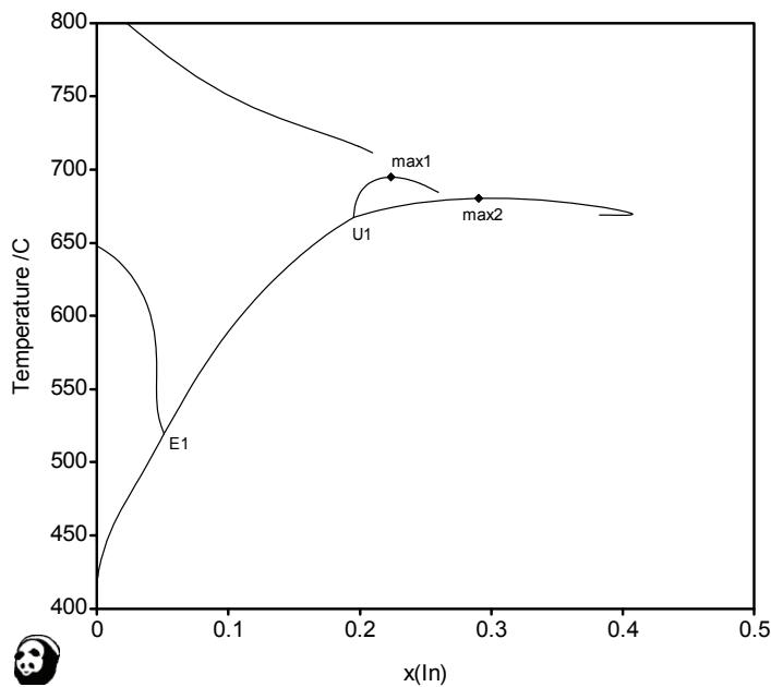
**Fig. 190:** Liquidus lines in the Cu-In-Sn system in the region of the high-temperature invariants projected onto the T- $x(\text{In})$  plane
