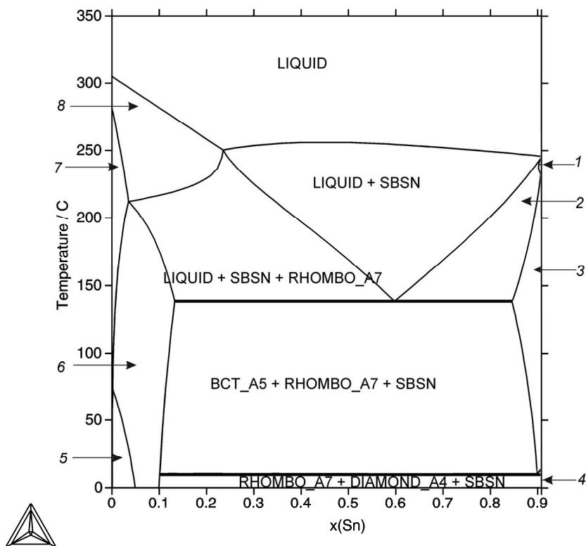
**Fig. 180:** Isopleth of the Bi-Sb-Sn system for 9 at% Sb
