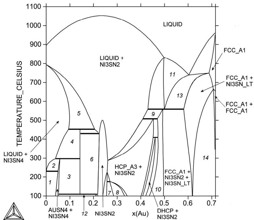
**Fig. 168:** Isopleth of the Au-Ni-Sn system for 28.6 at% Ni (around the ternary compound)
