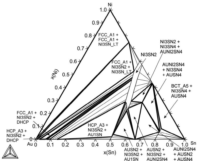
Fig. 163: Isothermal section at 200 °C
