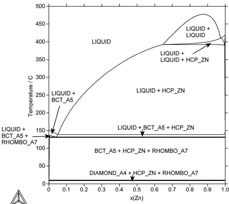
**Fig. 185:** Isopleth of the Bi-Sn-Zn system with the ratio Bi:Sn of 1:2
