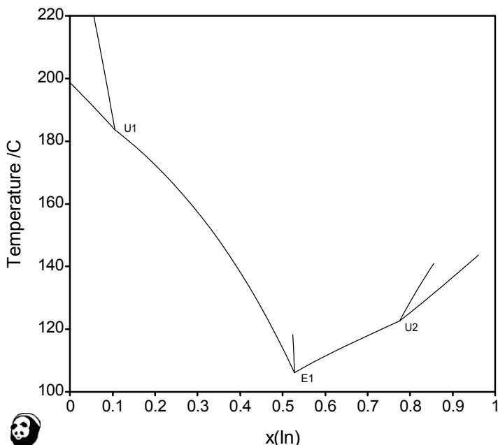
**Fig. 215:** Liquidus lines in the In-Sn-Zn system in the region of the low-temperature invariants projected onto the T- $x(\text{In})$  plane
