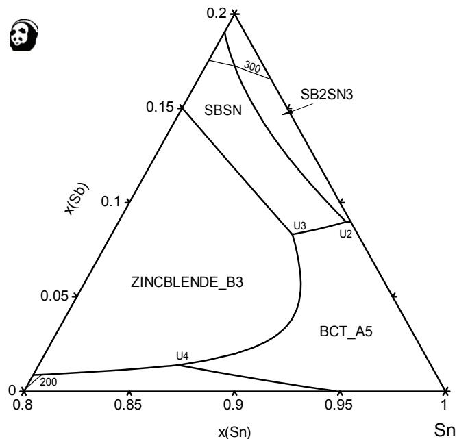
**Fig. 206:** Magnified view of the Sn-rich corner of the In-Sb-Sn system
