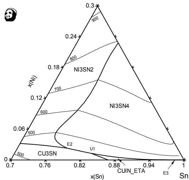
**Fig. 198:** Liquidus projection for the Sn rich corner of the Cu-Ni-Sn system
