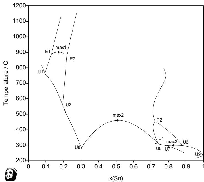
**Fig. 161:** Liquidus lines in the Au-Ni-Sn system projected onto the T-
