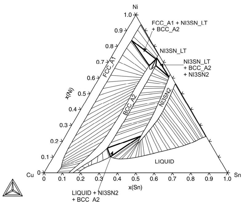
**Fig. 200:** Isothermal section at 800 °C
