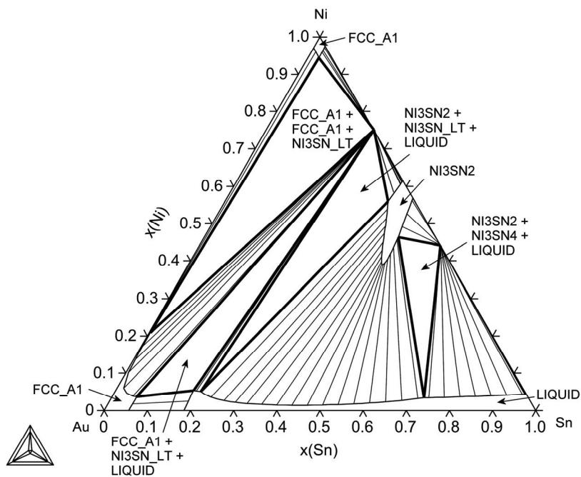
**Fig. 165:** Isothermal section at 600 °C
