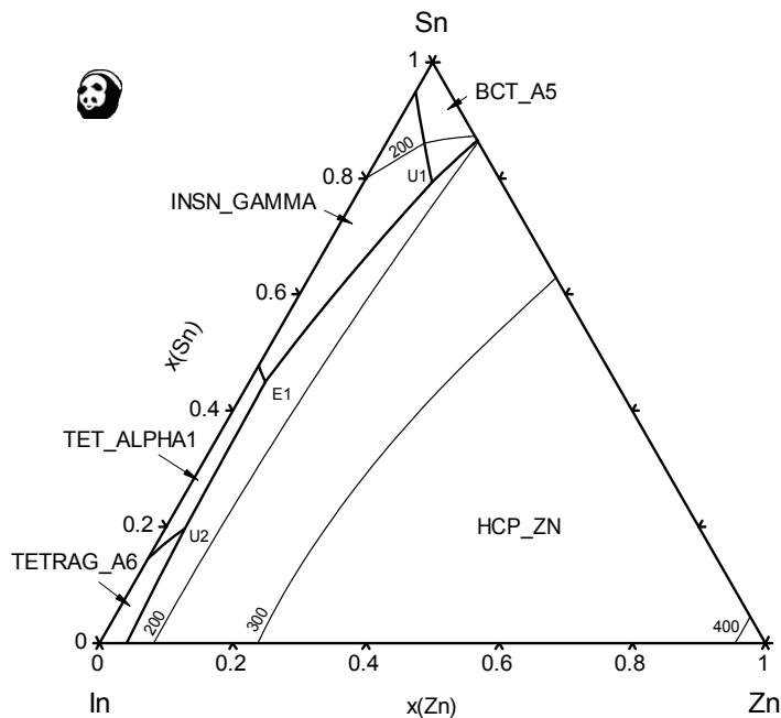
**Fig. 214:** Liquidus projection of the In-Sn-Zn system
