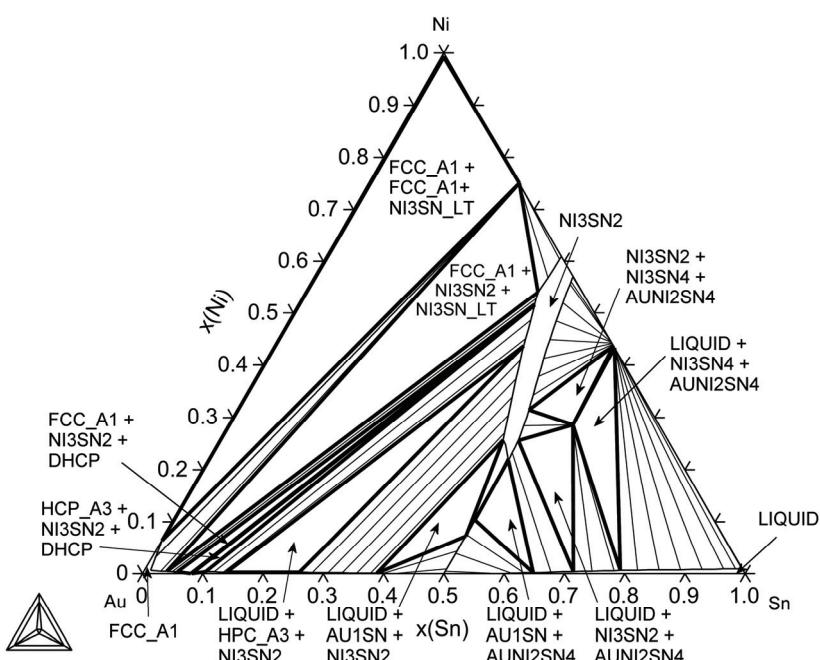
Fig. 164: Isothermal section at 400 °C
