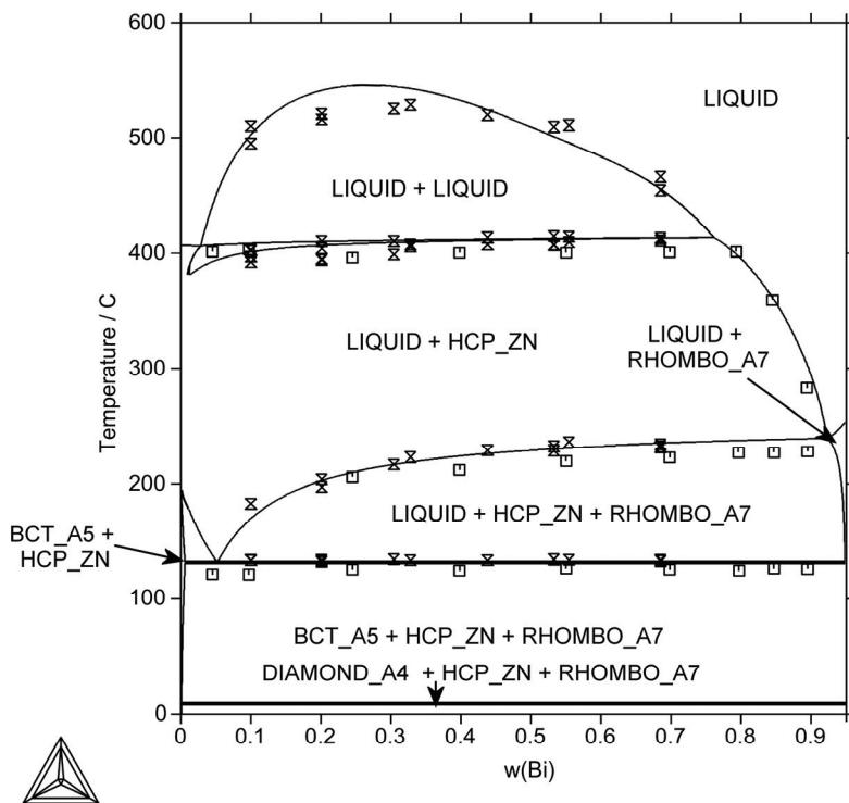
**Fig. 186:** Isopleth of the Bi-Sn-Zn system for 5 wt. % Sn (compared with exp. data from [23Muz] - □ and [07Bra] - ×)
