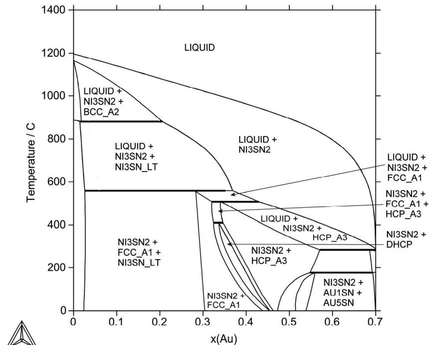
**Fig. 167:** Isopleth of the Au-Ni-Sn system for 30 at% Sn
