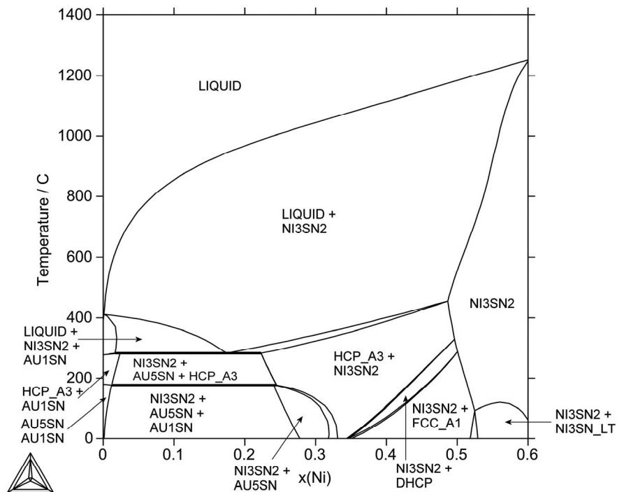
**Fig. 166:** Isopleth of the Au-Ni-Sn system for 40 at% Sn (close to the invariant point U8)
