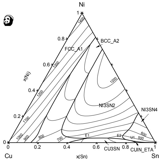
**Fig. 197:** Liquidus projection of the Cu-Ni-Sn system
