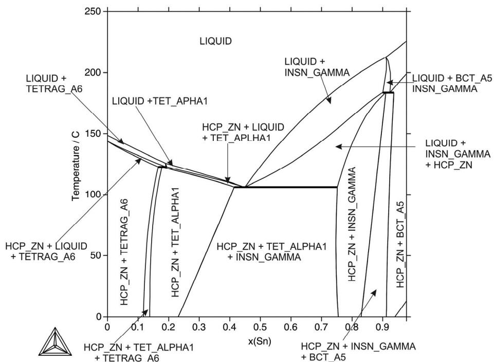
**Fig. 218:** Isopleth of the In-Sn-Zn system for 2.4 at% Zn (near the invariant point E1)
