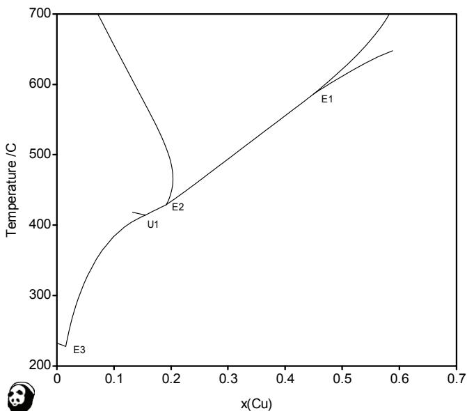
**Fig. 199:** Liquidus lines in the Cu-Ni-Sn system in the region of the low-temperature invariants projected onto the T- $x(\text{Cu})$  plane
