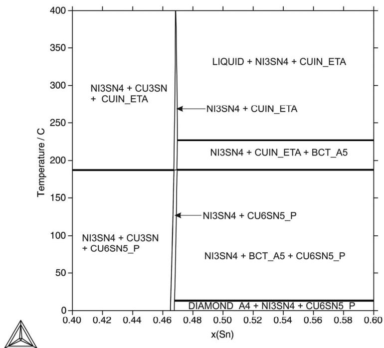
**Fig. 203:** Detail of the isopleths of the Cu-Ni-Sn system for 4.5 at% Ni
