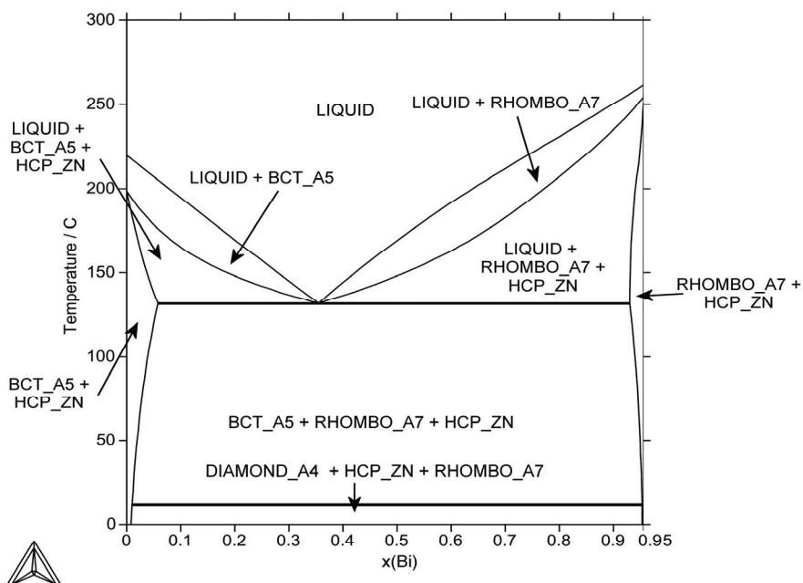
**Fig. 183:** Isopleth of the Bi-Sn-Zn system for 4.456 at% Zn (eutectic Zn concentration)
