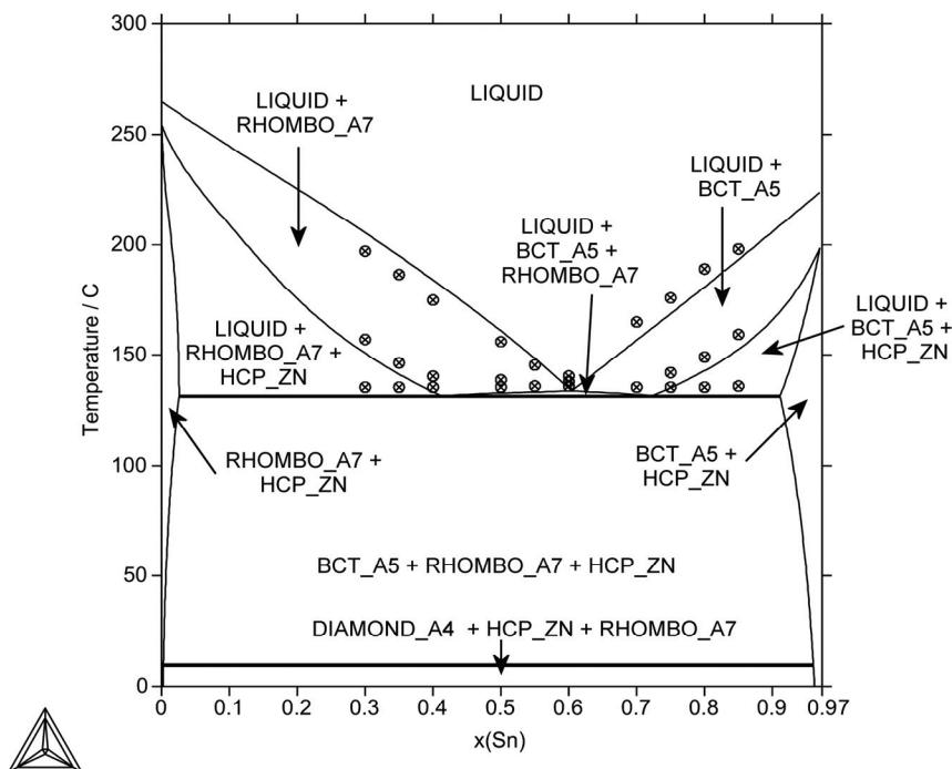
**Fig. 184:** Isopleth of the Bi-Sn-Zn system for 3 at% Zn (compared with exp. data from [06Lue])
