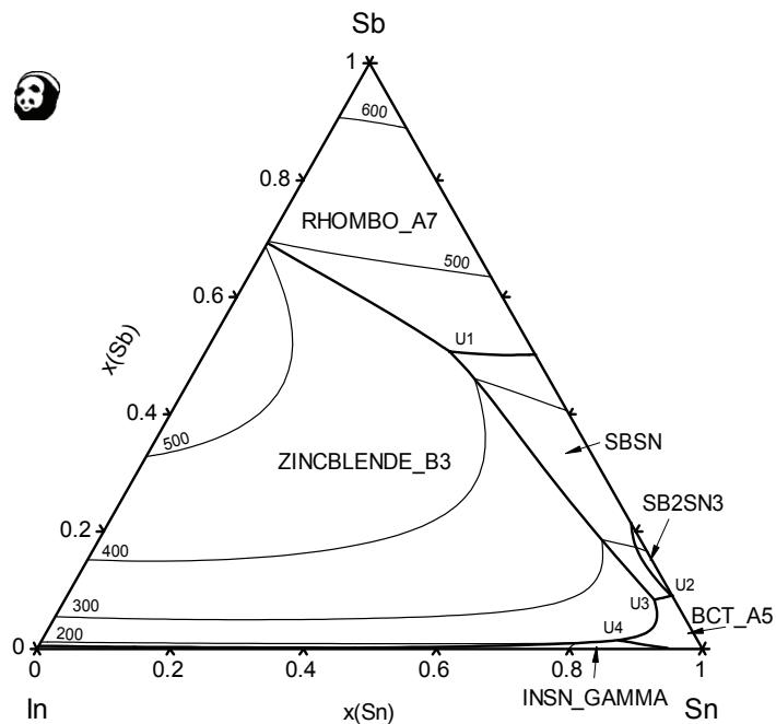
**Fig. 205:** Liquidus projection of the In-Sb-Sn system
