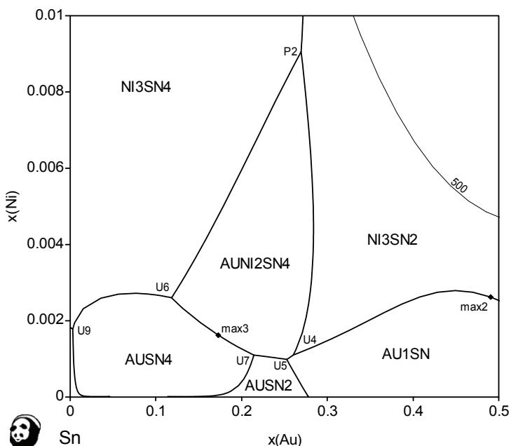
**Fig. 160:** Liquidus projection in the Sn-rich corner of the Au-Ni-Sn system
