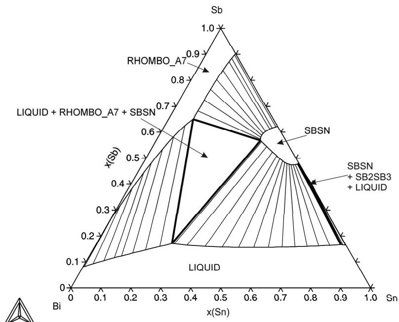
Fig. 177: Isothermal section at 300 °C
