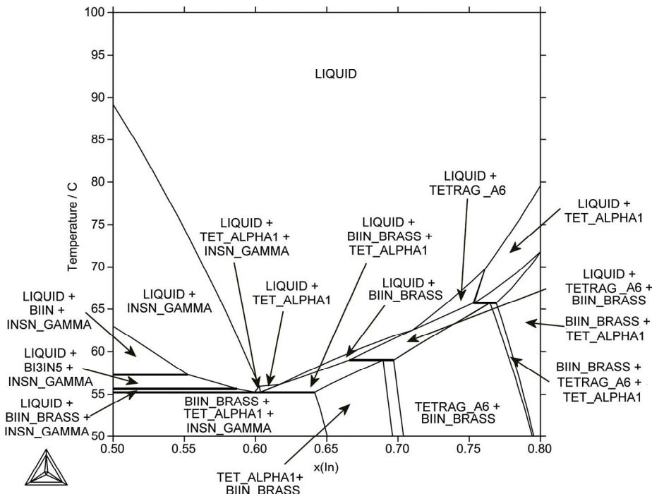
**Fig. 173:** Partial isopleth of the Bi-In-Sn system for 20 at% Bi
