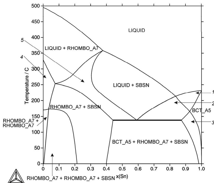
**Fig. 179:** Isopleth of the Bi-Sb-Sn system with the ratio Bi:Sb of 1:1
