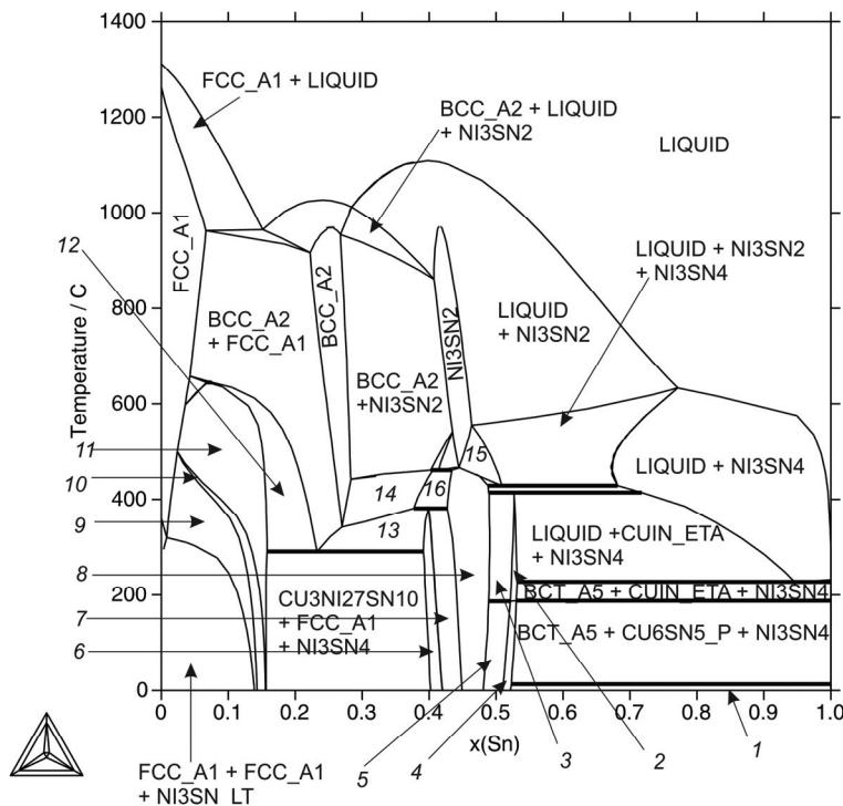
**Fig. 204:** Isopleth of the Cu-Ni-Sn system with the ratio Cu:Ni of 1:1
