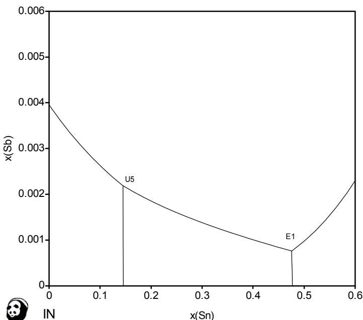
**Fig. 207:** Magnified view of the In-rich corner of the In-Sb-Sn system
