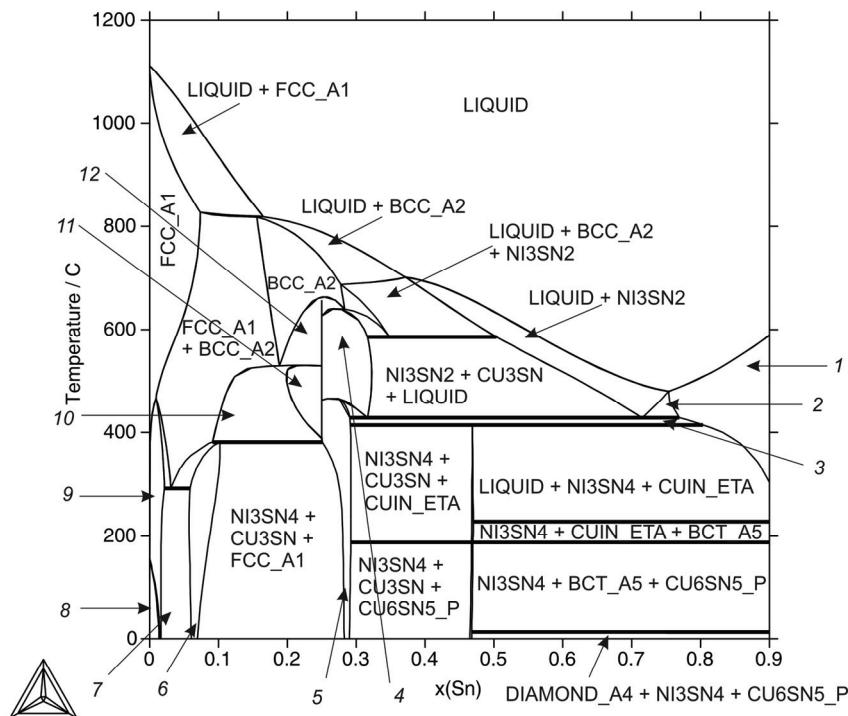
**Fig. 202:** Isopleth of the Cu-Ni-Sn system for 4.5 at% Ni
