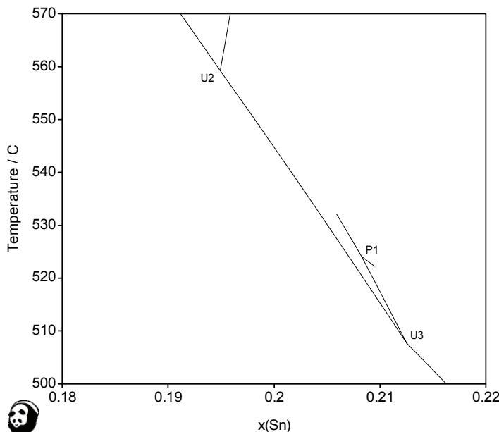
**Fig. 162:** Magnification of liquidus projection of the Au-Ni-Sn system on
