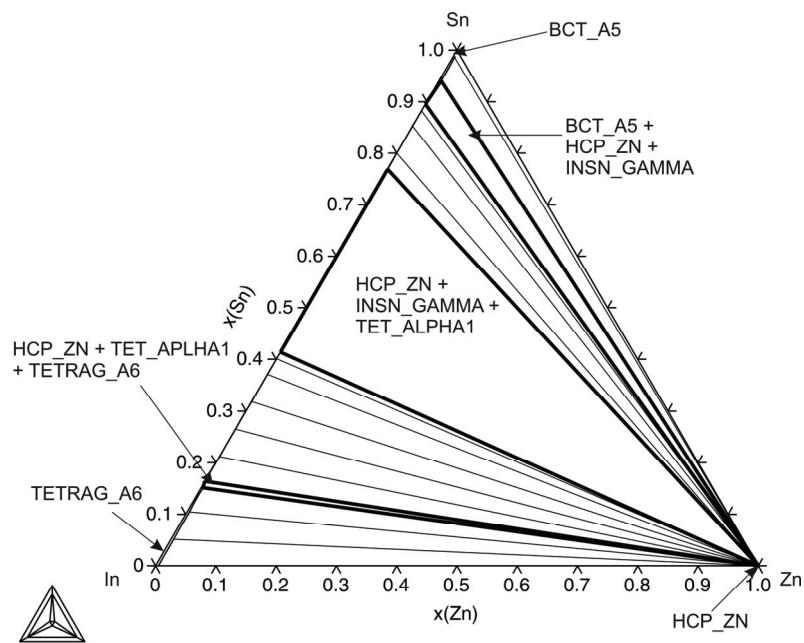
Fig. 216: Isothermal section at 100 °C
