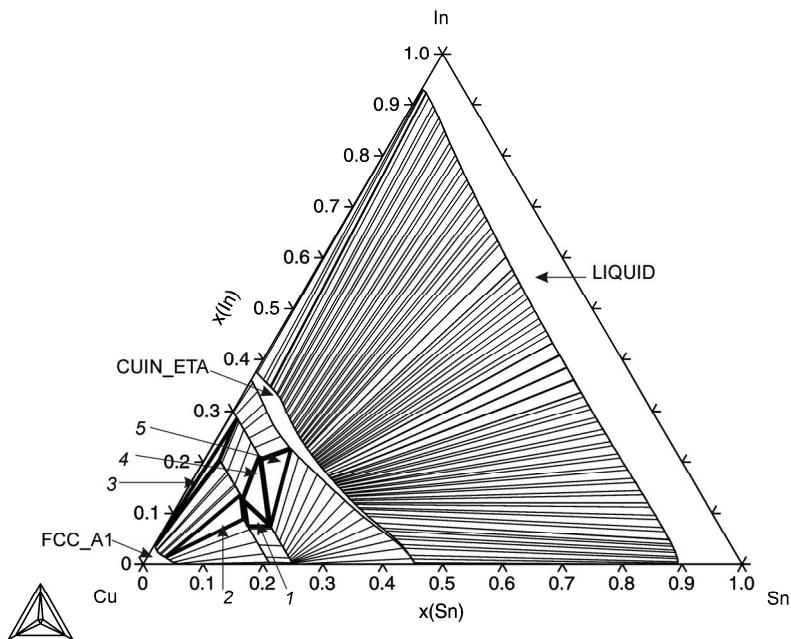
**Fig. 193:** Isothermal section at 400 °C
