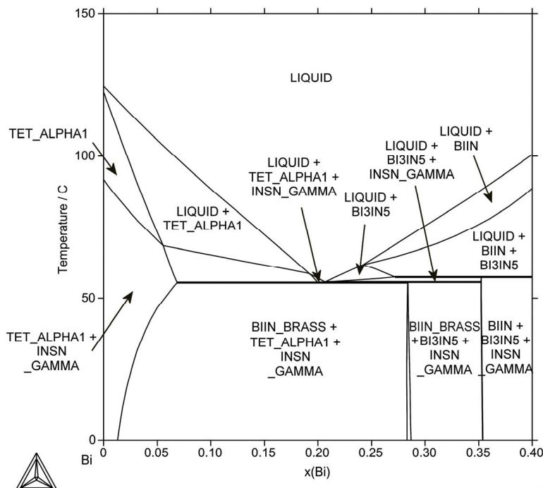
**Fig. 172:** Isopleth for 60 at% In (near the invariant points E1, U6)
