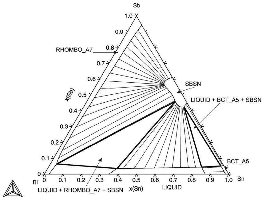
Fig. 176: Isothermal section at 200 °C
