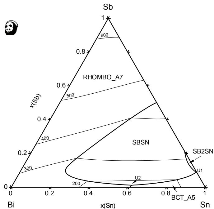
**Fig. 174:** Liquidus projection of the Bi-Sb-Sn system
