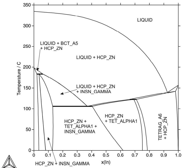
**Fig. 219:** Isopleth of the In-Sn-Zn system with the ratio Sn:Zn of 1:1
